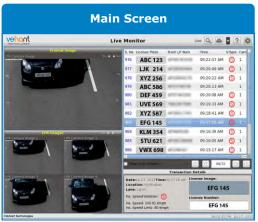
Main Screen displays the live transactional data of the vehicles passing through the lanes with four different frames. It displays the instantaneous speed, number plate of the vehicle, location and time.
