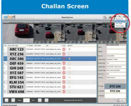
Challan Screen displays the list of speed violating vehicles as per user-defined criteria with details including instantaneous speed vehicle number plate, location and time stamp. The operator uses the information to validate and print the challan.
